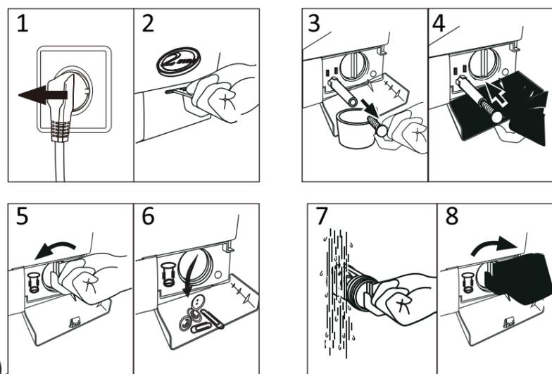
⚠ The filter must be in place, or it may lead to leakage.
