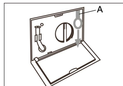
Not till then pull lever beneath service flap until door is unlocked by a gentle click.Afterwards refix all parts.
