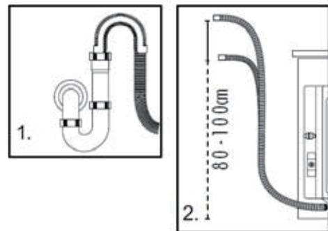
⚠ The drain hose should not be submerged in water and should be securely fixed and leak-free. If the drain hose is placed on the ground or if the pipe is at a height of less than 80cm, the washing machine will continuously drain while being filled (self-siphoning).
