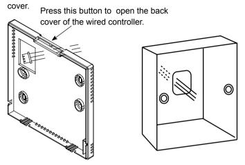
2. Fix back cover to the holder. After that, connect communication wire to CON1 port of wired controller. Finally put the front cover of wired controller to back cover to complete the installation.
