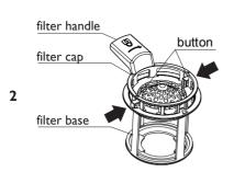
Twist the filter handle anti-clockwise to release. Lift to remove from the filter plate. Separate the filter cap from the base by pressing the release buttons and lifting. Remove the filter plate gently from the locating clips at the rear of the drain. Do not attempt to remove the filter by force as this may cause damage. Clean under hot water and rinse thoroughly.
