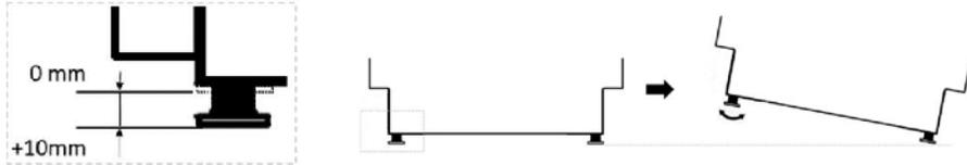
**IMPORTANT!** Cooker needs to be supported properly when tilted to avoid any possible hazard.
