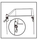
7. Make the middle hinge reverse the direction 180°C, then transfer it to the left property position. Make the middle hinge pin in the upper hole of the lower door, then tight the screws.
