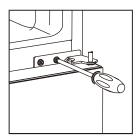
4. Laying down the refrigerator, take out the adjusting feet as below, then unscrew the lower hinge by cross screwdriver.
