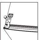
9. Take left hinge cover from accessary bag and install it with top hinge. Then install hole cover at right side.
