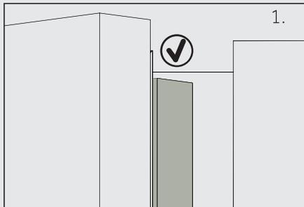
When you close the door, the vertical door beam on the fridge left door should be bent inside (1).
