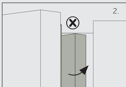
If you try to close the left door and the vertical door strip is unbent (2), you should bend it firstly, otherwise the door strip will hit the Beam Track or right door. Thus a damage to the door slip or a leak will occur.
