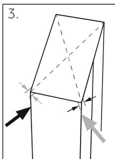
3. The stability can be checked by alternately bumping on the diagonals. The slightly swaying should be the same in both directions. Otherwise the frame can warp; possible leaking door seals are the result. A low tendency to the rear facilitates the closing of the doors.
