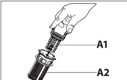
2. To disassemble the filter **A** press the latches and unplug **A1** from **A2**.
