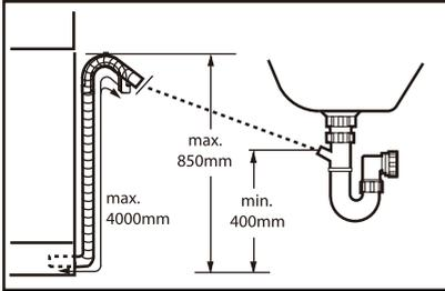
Fix the water drain hose properly to the piping. The hose has to reach at one point a height between 400 and 850 mm above the appliance bottom line!
