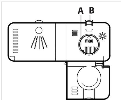
1. Press the release button (**B**) to open the lid.
