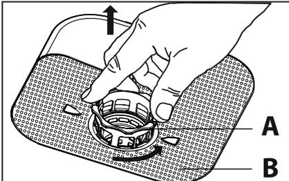
1. Turn the filter **A** anticlockwise and remove it.
