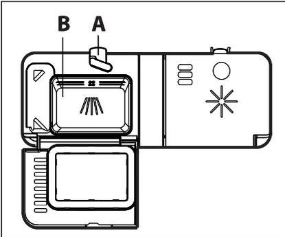
1. If the lid is closed press the release button **(A)** to open the lid.
