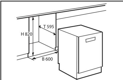
1. The dimensions of the recess should at least agree with the dimensions in the figure.
