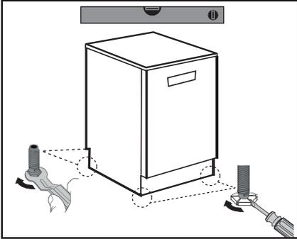
1. Install the appliance on solid ground. Adjust accurately all feet to get a firm, horizontal position.
