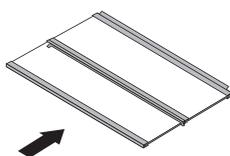
The front of the foldaway shelf can slide in backwards. This allows the storing of larger items on the shelf below.
