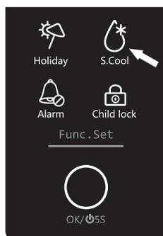
Switch on the Super cooling function if larger quantity of food should be stored (for example after the purchase) or if you want to cool drinks quickly. The Super cooling function accelerates the cooling of fresh food and protects the goods already stored from undesirable warming. The factory setting temperature is + 2 ° C.
