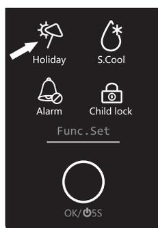
This function sets the refrigerator temperature permanently to 17°C. So you have the possibility to let the empty appliance closed without causing a smell or mold during a long absence (E.g. holiday).
