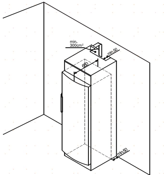
The freezer can be inserted into a row of kitchen units. To match the freezer to the height of row of the units, a suitable stack cabinet can be added. When inserting the freezer into a row of standard kitchen units (max. depth 580 mm), the appliance can be installed directly next to the kitchen unit. The freezer door projects relative to the front of the kitchen units by 34mm at the side and by 55mm in the middle of the freezer. It can be opened and closed perfectly as a result.
