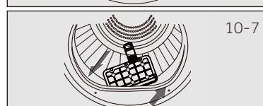
5. Reinstall the sponge into the condenser filter and put the filter back into the duct
