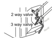
7. To prevent the gas leakage, turn the service ports cap, the valve rodis cap for 2-way valve and 3-way's a little more than the point where the torque increases suddenly.
