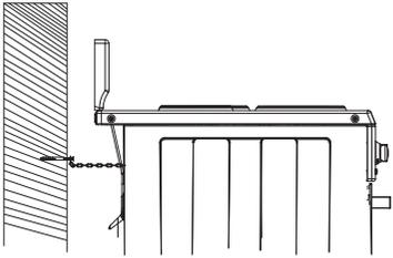
Anti tilt chains are located at the rear of the appliance and must be secured to the wall behind the appliance to prevent accidental tipping/tilting. The chain length must be as short as practicable to avoid appliance tilting forward and also diagonal to avoid appliance moving sideways.
