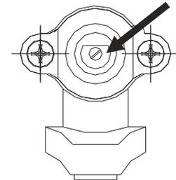
Knobs should be adjusted with the burner switched on and set to the economical flame position, using an adjustment screwdriver of the 2.5mm size.
