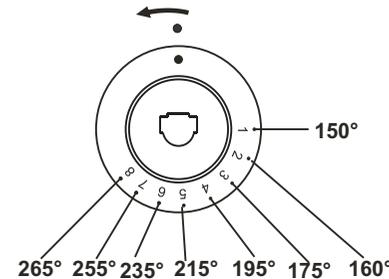
Oven is equipped with gas valve with temperature regulator and anti-outflow protection. To ignite the oven, as in the description below, keep down the pressed knob during about 3 s, this is the time necessary to warm the sensor and to make the protection function. If the flame goes out, repeat ignition operations after a lapse of 3 sec. if the flame does not start burning within 10 sec., repeat the ignition operation after lapse of about 1 min, i.e. after the oven ventilation.
