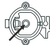
Exchange of a burner nozzle : unscrew the nozzle with special socket spanner No 7 and replace with a new one according to a type of gas (see tables)
