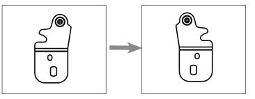
8. Refit the bracket fitting the bottom hinge pin. Replace both adjustable feet. Transfer the lower door to the property position.
