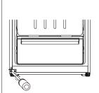
9. Make the middle hinge reverse the direction 180°C, then transfer it to the left property position. Make the middle hinge pin in the upper hole of the lower door, then tight the bolts.
