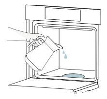
**2.** Pour 100 ml of water into the base of the oven.
