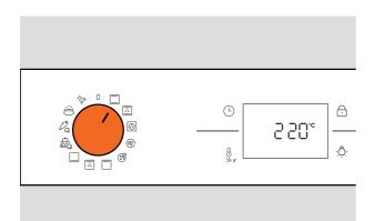
1. Turn the FUNCTION DIAL to select the desired cooking function. This turns the oven ON. The default temperature for the function will show on the display.
