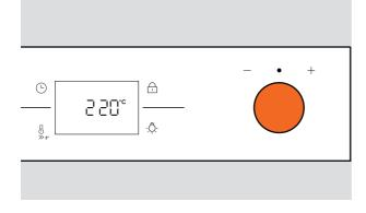
**2.** Turn the **CONTROL DIAL** to adjust the temperature.
