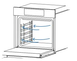
**3.** Push the racks back into the side of the oven to refit.
