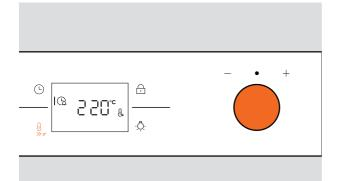
2. To adjust the temperature while the timer is on, press  $\frac{A}{2}$ , to access TEMPERATURE mode, then turn the control dial to adjust the temperature.
