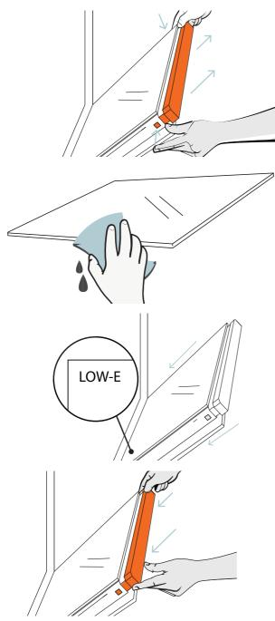
1. Shut the door halfway, then press the buttons on both sides of the door at the same time to release the cover on top of the door.
