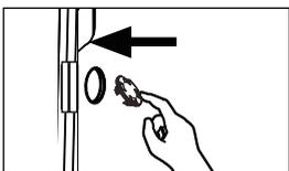
2. Fill the transportation bolt holes with blanking plugs.
