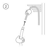
If additional length of hose is required, a hose extender is included with your dryer, uncoil the extender and plug the 2 hoses together.
