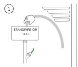
Unclip the drain hose on the back of the product and connect it to a standpipe or tub.
