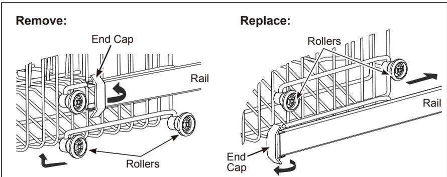
1. Fully extend the upper rack and rotate open the two plastic end caps on the front of the rails.
