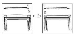
8 Install the upper door, fix the upper door hinge  $% \left( 1\right) =\left( 1\right) +\left( 1\right)$
