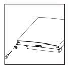
Use a flat-bladed screwdriver to pryopen the upper door sleeve and corner plastic cover. Turn the door sleeve 180° then put it backon the upper door. Turn the plastic cover 180° then put it to opposite side where the top hinge bracket will be fixed.
