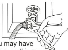
2. Connect the water inlet hose to the water faucet. You may have to use pliers to tighten the coupling. Do not over tighten as this may cause damage to the valve or hose fittings.
