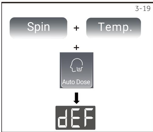
Quick method to deactivate preferred settings for all cycles, just select the " Ultra Quick" cycle, then press the "Spin", "Temp." and " Auto dose " buttons (Fig. 3-19) simultaneously for 3 seconds, the screen will display **dEF** , and all cycles will go back to its default settings.
