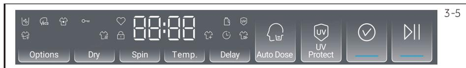
After selecting a cycle, users can also select different functions based on their needs by pressing on the function buttons (Fig. 3-5).
