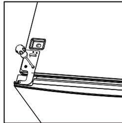
9. Take left hinge cover from accessory bag and install it with top hinge. Then install hole cover at right side.
